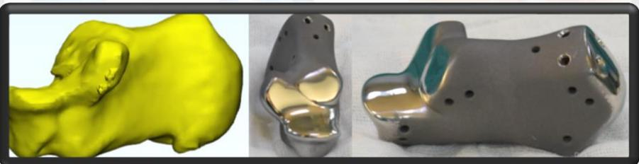
3D printed calcaneal prosthesis
