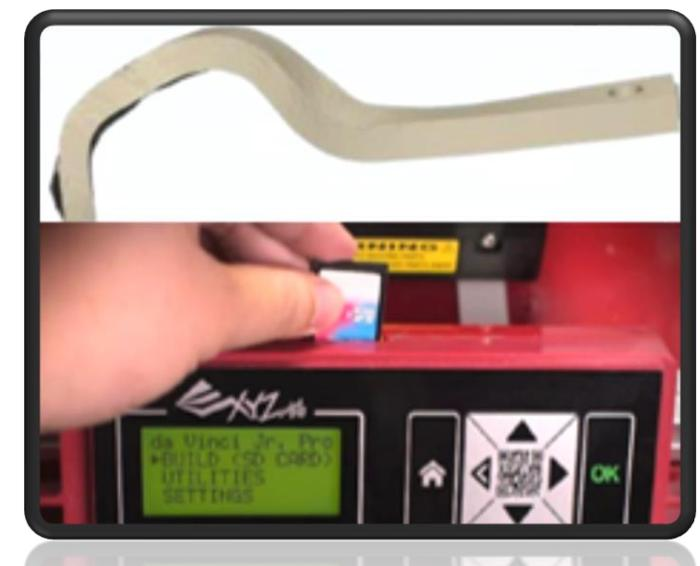
Jig file transferred to 3D printer
